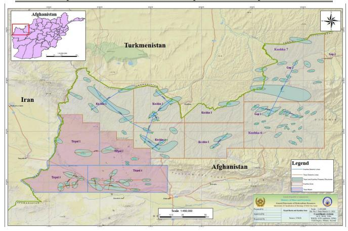
Annex B: Prospective Structures in the Kushka Tirpul Basin with Proposed Seismic Lines
